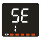
EXIT Menu: You can exit the setting menu by pressing M for a long while in any setting menu. Besides, you can exit the setting menu automatically by pressing M for a short while and switching all the setting items.
