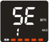
SET2(speed limited): When in SET2, the factory default limited speed of the instrument is 25km/h. The effective limited speed ranges from 10 km/h to 50km/h by pressing +/-. It doesn't work if over the range. You can quit the interface by pressing M for a short while to set the next item or pressing M for a long while.
